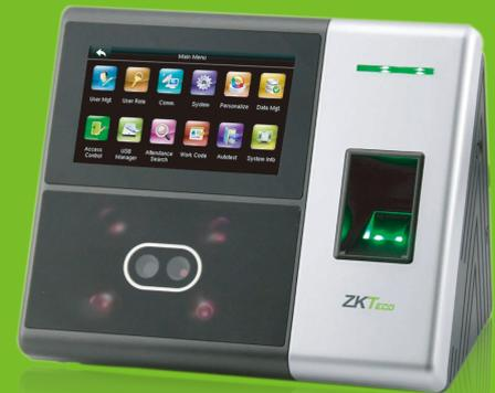
ZKTeco's newly released SFace900 Semi-Outdoor Multi-Biometric Time Attendance & Access Control Terminal which supports 3,000 face templates, 4,000 fingerprint templates and 10,000 cards.
