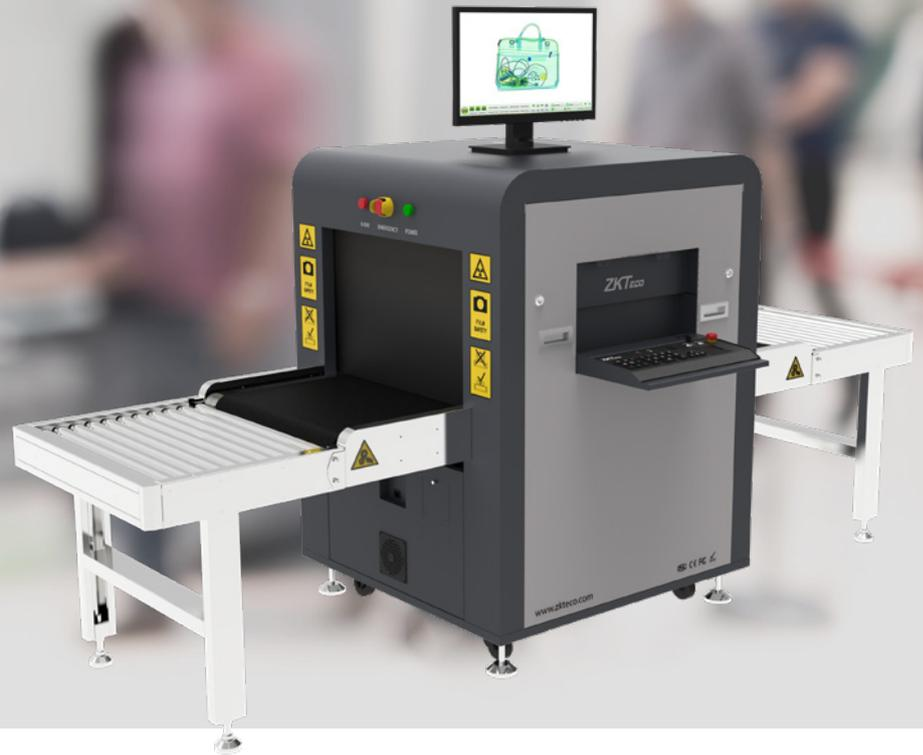
ZKX6040 is an advanced dual-energy X-ray baggage inspection assistant whose capabilities include penetration of up to 35mm of steel with an optimized algorithm. Its tunnel opening is as large as 600 mm by 400 mm.
